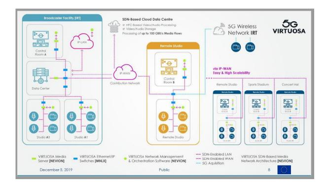
The plan for project VIRTUOSA is to build a real-life live production set-up combining broadcast facilities and remote studios connected by IP networks (both LAN and WAN), combined with remote live contributions from cameras connected via a 5G network.
